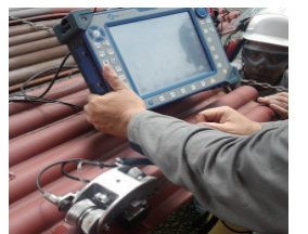
Corrosion Inspection of Boiler Water Wall
