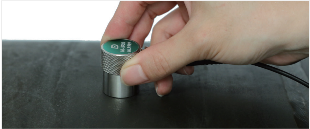
A single crystal transducer, sound wave vertical incidence and direct contact.
