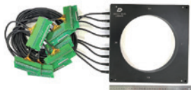
Circular array probe
